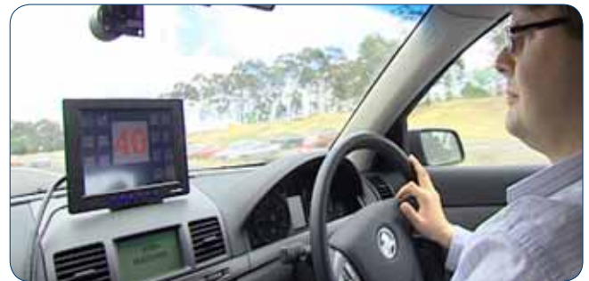
The Speed Sign Recognition System at work at Latrobe University
